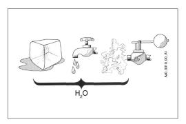
taking a substance from the vapour to the liquid phase the transition process is called condensing and when taking it further to the solid phase the transition process is called freezing (solidification).
