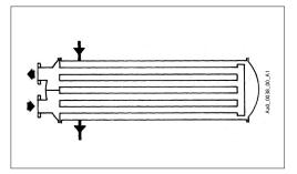
water so that it circulates several times through the condenser. As a rule, the water becomes heated 5-10 °C when it has passed through a condenser.
